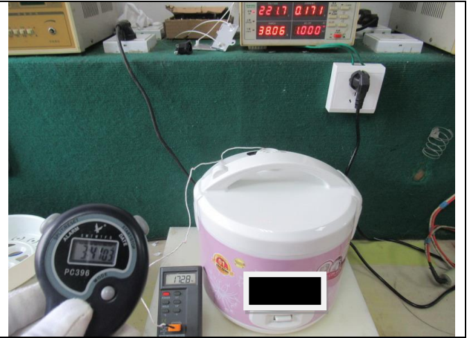
Dry burning test (Temperature limiter)
