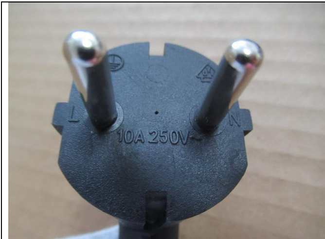
N1. The plug with 10A 250V" instead of "16A 250V" shown on the customer profile.
