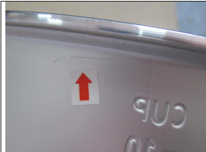
Minor-Scratch mark on the inner pot
