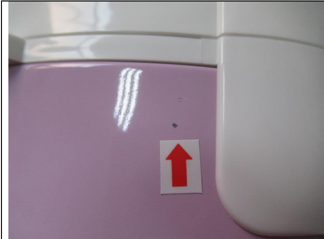
Major-Impurity mark in the coating of housing
