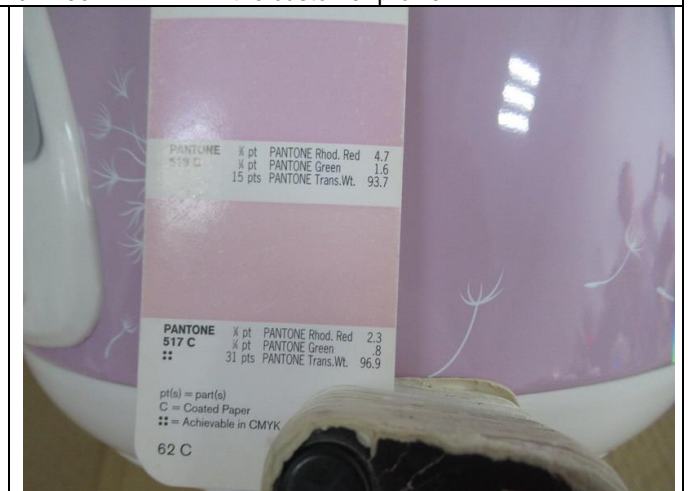
N5. For pantone check, found color of housing was different from Pantone 517C.
