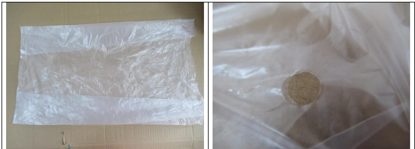
F3. The polybag without suffocation warning words, but air hole on polybag was found.
