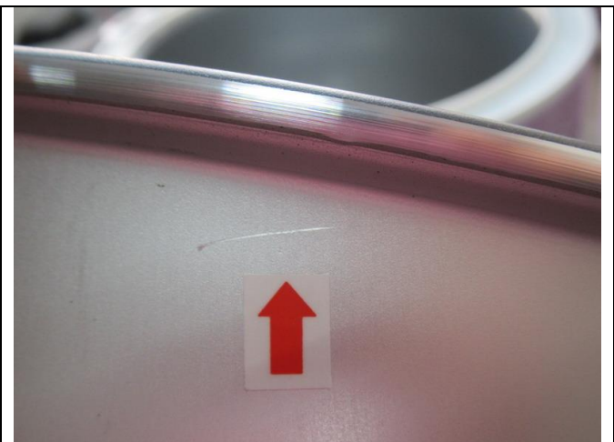
Minor-Scratch mark on the inner pot
