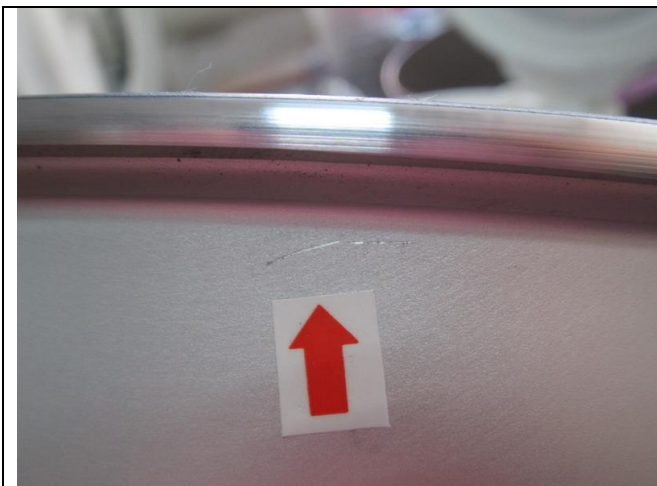
Minor-Scratch mark on the inner pot
