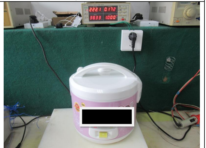
Dry burning test (Self-reset thermal cut-out)
